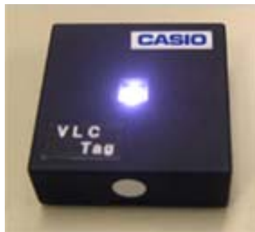
Photo 4 Light source: Chip LED with button cell, 3x3x1 cm
