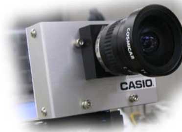
Photo 5 Sensor module with USB port, about 10x6x1.5 cm
