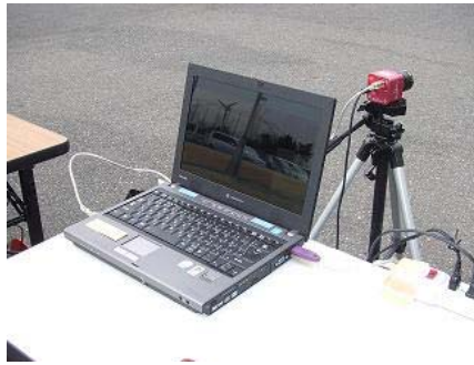
Photo 3. Visible Light Communications receiver (CMOS camera and inbound processing device)
